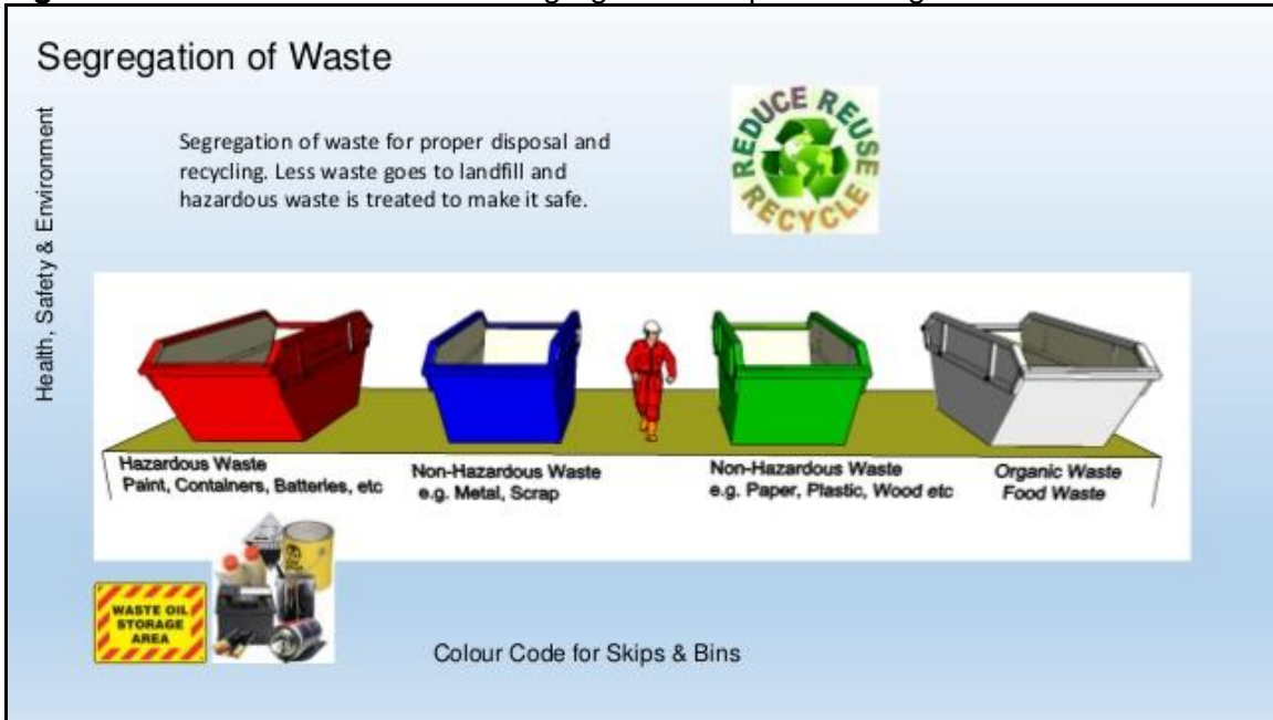
Figure 1 Construction Waste segregation compound design
